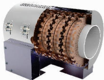
In a ceramic band heater, nickel-chrome wire is embedded in a flexible outer wall made of special, interlocking ceramic tiles (KNUCKLES), which are assembled like a brick wall. A ceramic fiber insulating mat and a stainless Steel/Aluminised Steel jacket cover this assembly. This construction prevents heat loss and reduces electrical consumption by 20%.
