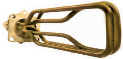
Tubular heating element consists of a resistant nickel chromium wire type 80/20 inserted into a protective metal tube (outer sheath) filled with high purity electro-melt Magnesium oxide (MgO). The assembly will be compacted by rolling/swaging process to ensure excellent heat transfer. Each edge of the sheathed component consists of a non-heating zone, where the electrical connection is made.
