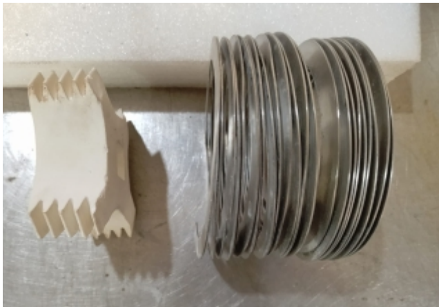
Fig:78 Ceramic Spacer (left) & Circular flat Heating Element (right) [1]
