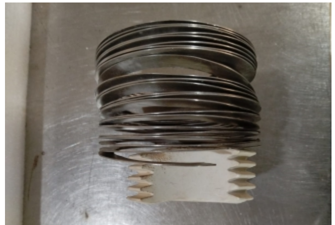
Fig:79 Ceramic Spacer & Circular flat Heating Element [2]
