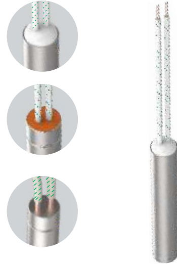
In heaters over 3 " long the leads make a connection with the power pins in a short unheated section.
